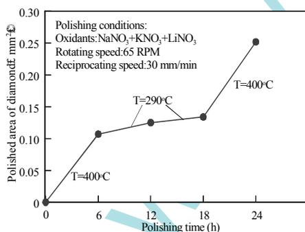
Fig.6 Polishing time versus polished area of diamond
