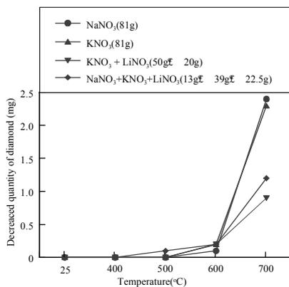
Fig.3 Static oxidation of diamond in different oxidizing agents and temperature
