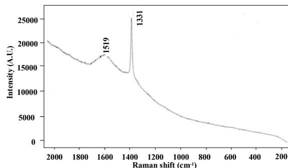
Fig.7 Raman spectrum of the diamond polished by mechanochemical method
