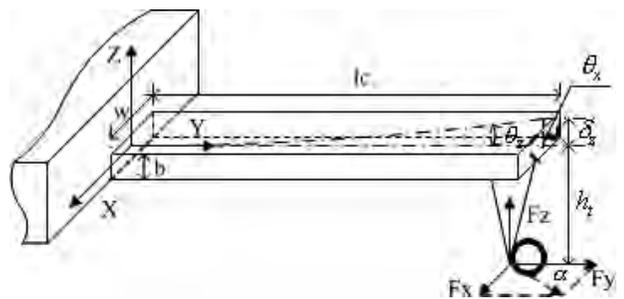
Fig. 1. Model of 3D nano forces dependent on cantilever deflections.
