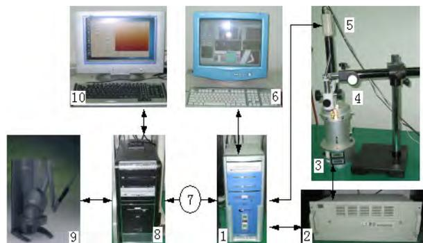
Fig. 7. The configuration of AFM based robotic nanomanipulation system, (1) AFM control computer, (2) CSPM 2000wet controller, (3) AFM head, (4) optical microscope, (5) CCD camera, (6) monitor for imaging and optical vision, (7) Ethernet device, (8) haptic device control computer, (9) 3-DOF haptic device, (10) monitor for visual interface.
