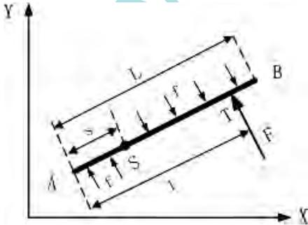
Fig. 6. Rotation motion of MWCNT acted by the probe.
