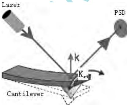
Fig. 2. Cantilever deflections measured by PSD.
