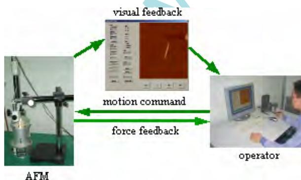
Fig. 8. Robotic nanomanipulation mode with real-time force and visual information feedback.
