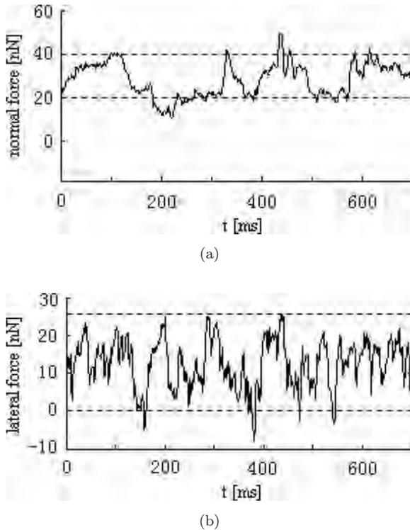
Fig. 10. Nano forces in the first push (a) normal force, (b) lateral force.
