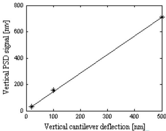
Fig. 4. The dependent curve of vertical cantilever deflection on vertical PSD signal.
