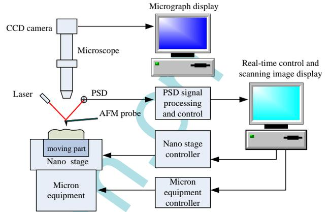
Fig. 4. Structure of the AFM system based on nano positioning stage.
