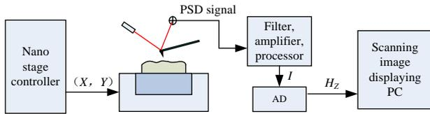
Fig. 5. Control scheme for constant height scanning mode.
