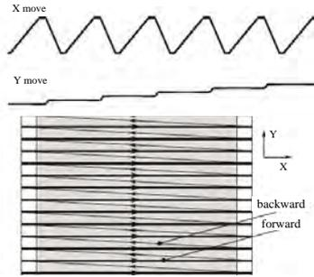
Fig. 2. Scanning motion of the stage implemented by the cooperating motions of the X and Y actuators.
