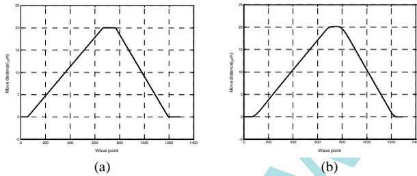
Fig. 3. Moving track of the actuator at low and high speed: (a) moving at low speed (b) moving at high speed.
