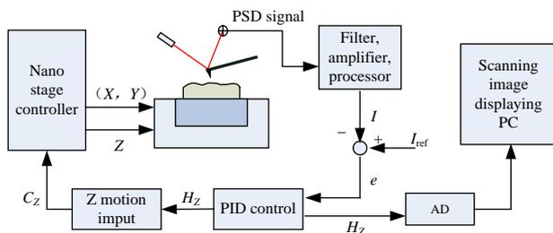
Fig. 6. Control scheme for constant force scanning mode.
