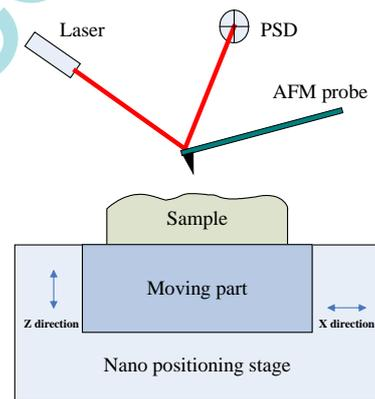
Fig. 1. Basic structure of the AFM.
