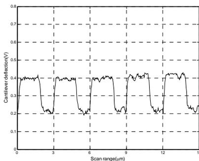
Fig. 9. Profile of the standard grating.
