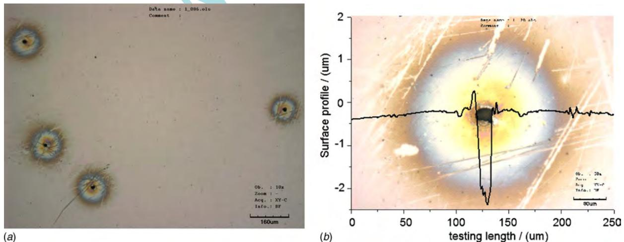
Fig. 2 (a) Pits scattered on the surface and (b) surface profile of the erosion pit tested by confocal laser scanning microscope; the uncertainty of the measured data is  $0.01 \mu\text{m}$  according to the precision of the microscope
