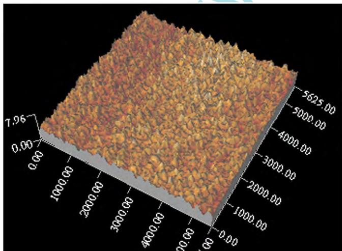
Fig. 4. The morphology of amine functional film on p-Si (100) surface (Ar 100 sccm, 2000 Pa, 30 min, DC = 30%).
