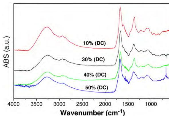
**Fig. 2.** FTIR spectra of the plasma polymerization amine-containing functional films in different duty cycles (Ar 100 sccm, 2000 Pa, 30 min, 20 W).
