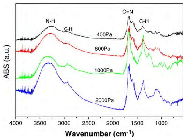
**Fig. 1.** FTIR spectra of the plasma polymerization amine-containing functional films in different gas pressures (Ar 100 sccm, 5 W, 30 min, duty cycle (DC) = 30%).
