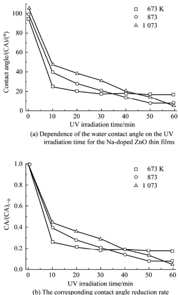
Fig.4 Dependence of the water contact angle on the UV irradiation time for the Na-doped ZnO thin films and the corresponding contact angle reduction rate  $(CA/(CA)_{t=0})$  ( $CA)_{t=0}$  is contact angle at start time.
