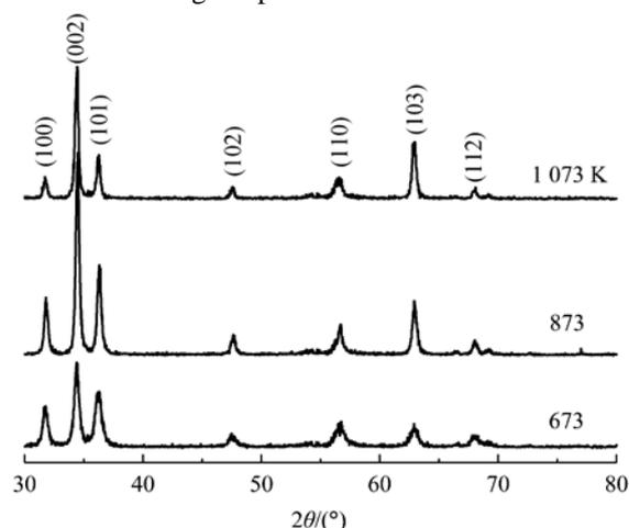
Fig.1 XRD patterns of Na-doped ZnO thin films annealed at different temperatures for 60 min
