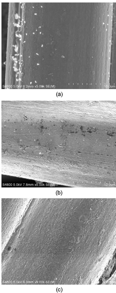
Figure 4. SEM images of sample 4 (a) plasma treatment, (b) Ag coated for 30 min, and (c) Ag coated for 60 min.
