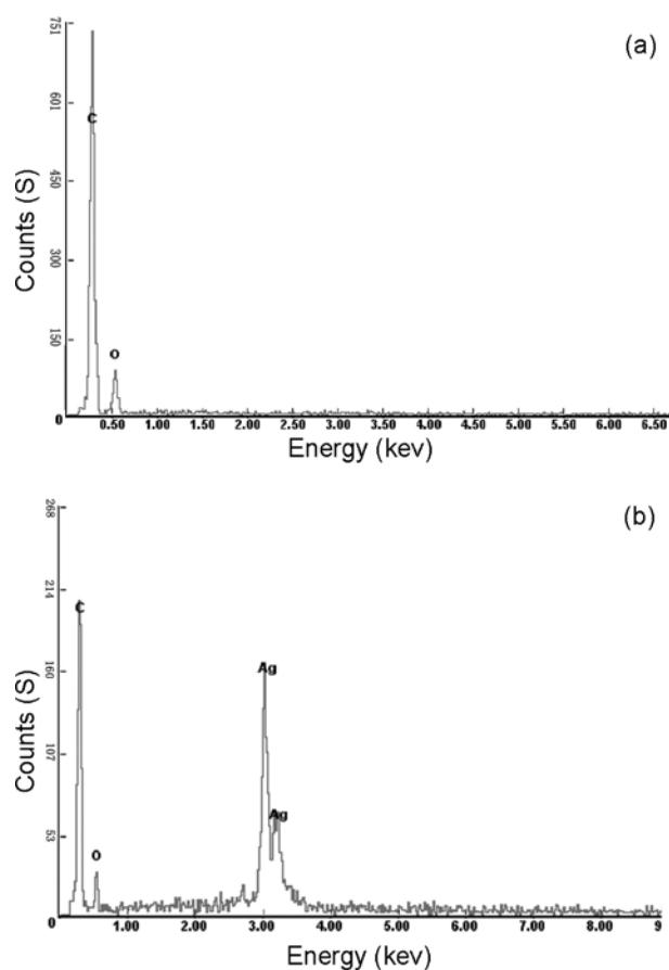
Figure 5. EDX spectra of samples (a) raw sample and (b) samper 1 coating 30 min.
