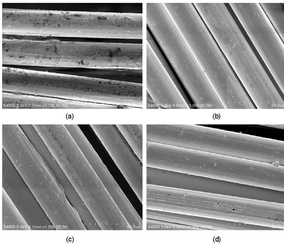
Figure 2. SEM images of sputtered Vectran yarns (a) raw sample : coated for 30 min, (b) sample 1: coated for 30 min, (c) sample 2: coated for 30 min, and (d) sample 3: coated for 30 min.
