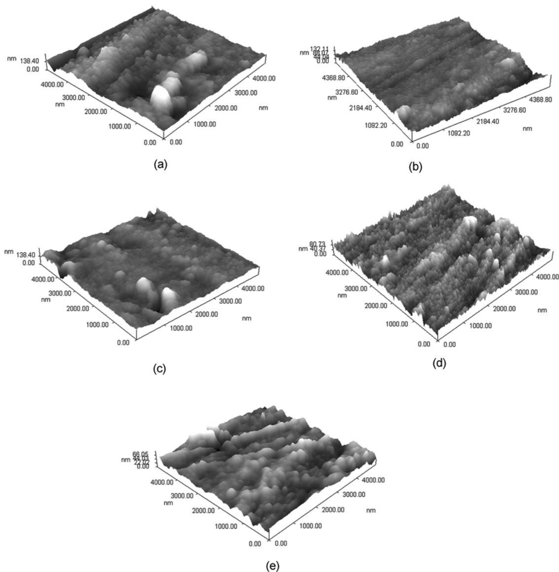
**Figure 3.** AFM images of sputtered Vectran yarns (a) raw sample: coated for 30 min, (b) sample 1: coated for 30 min, (c) sample 2: coated for 30 min, (d) sample 3: coated for 30 min, and (e) sample 4: coated for 30 min.
