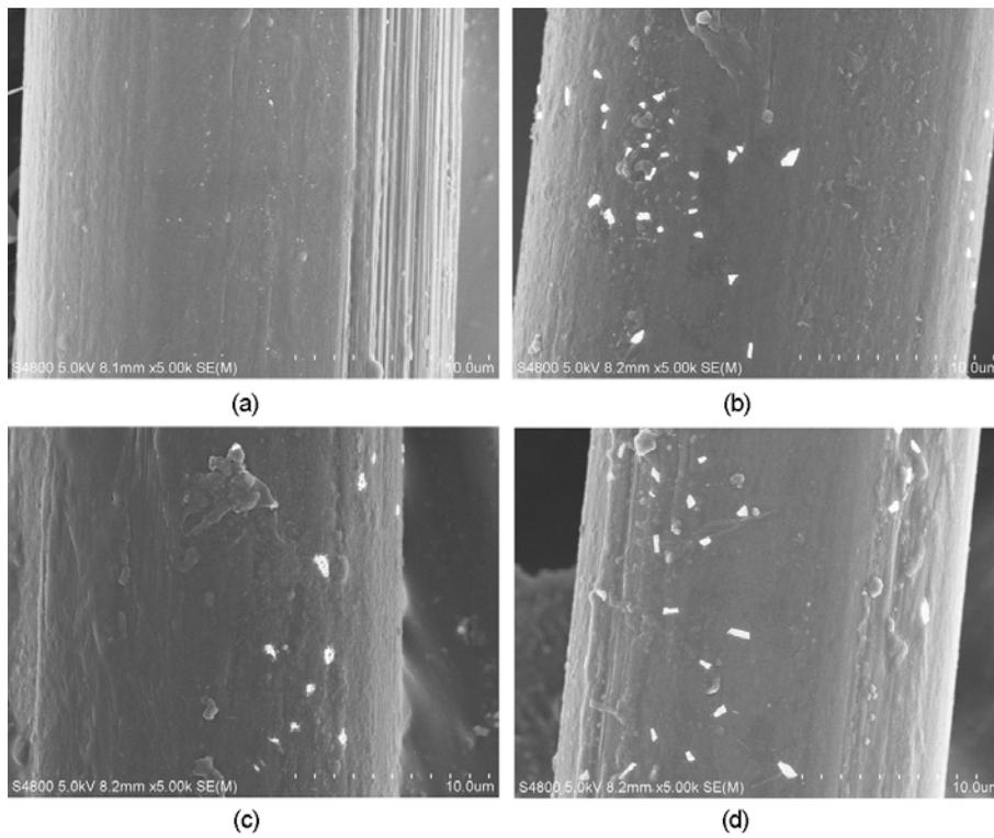
Figure 1. SEM images of plasma treated Vectran yarns (a) raw sample, (b) sample 1, (c) sample 2, and (d) sample 3.
