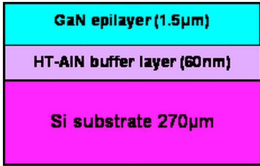
Fig. 1. Schematic view of GaN/Si(111) with the HT-AlN buffer layer.
