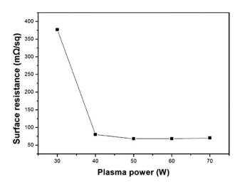
**Figure 6** Effects of the plasma power on the conductivity (vacuum degree = 30 Pa, pretreatment time = 1 min, CuSO<sub>4</sub> concentration = 20 g/L, reaction temperature =  $43^{\circ}$ C).
