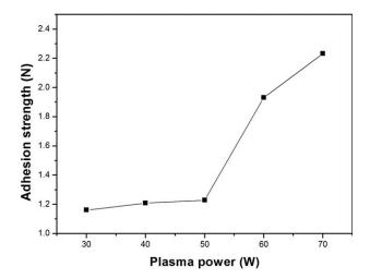
Figure 7 Effects of the plasma power on the adhesion strength.
