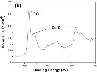
**Figure 3** XPS spectra of the copper-deposited PP fibers: (a) C1s, O1s, and Cu2p3 and (b) Cu2p3.
