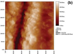
**Figure 2** AFM images of the coated fibers: (a) 8000 nm  $\times$  8000 nm and (b) 3000 nm  $\times$  3000 nm. [Color figure can be viewed in the online issue, which is available at www.interscience.wiley.com.]
