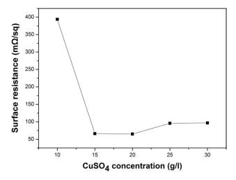
**Figure 4** Effects of the  $CuSO_4$  concentration on the surface resistance (vacuum degree = 30 Pa, reaction power = 50 W, pretreatment time = 1 min, reaction temperature =  $38^{\circ}C$ ).
