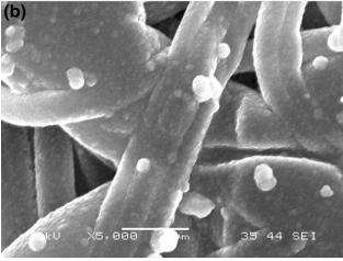
**Figure 1** SEM images of the PP nonwovens: (a) uncoated and (b) copper-coated.
