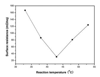
**Figure 5** Effects of the reaction temperature on the surface resistance (vacuum degree = 30 Pa, reaction power = 50 W, pretreatment time = 1 min, CuSO<sub>4</sub> concentration = 20 g/L).
