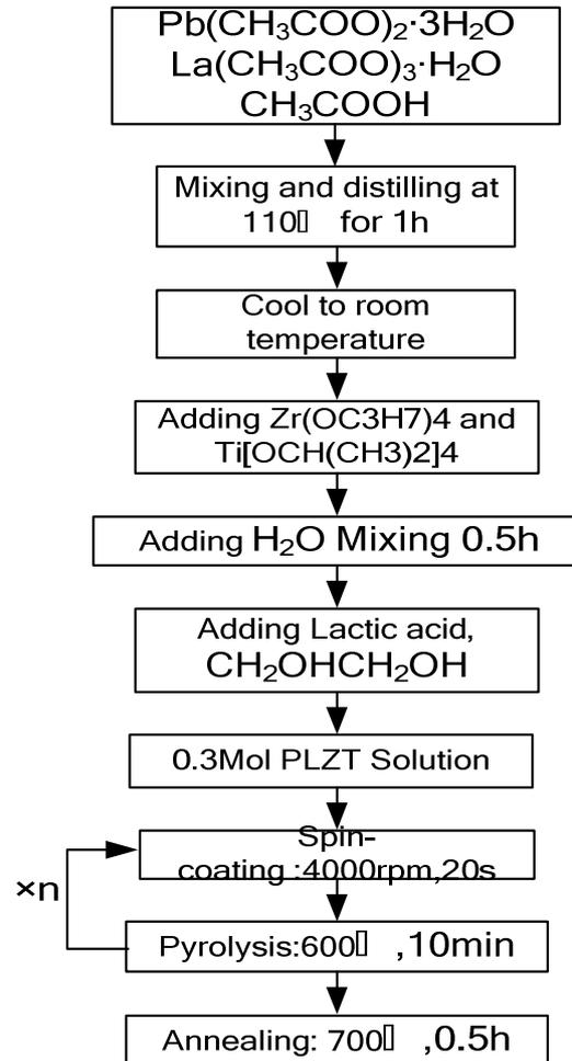
Fig. 1 Flow diagram of sol-gel processing for PLZT films
