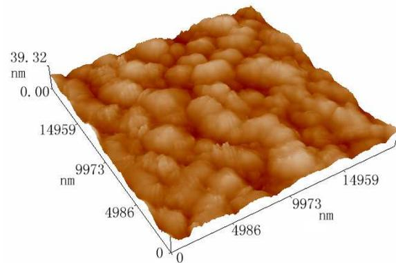
Fig.4 AFM surface morphology of PLZT antiferroelectric thick films
