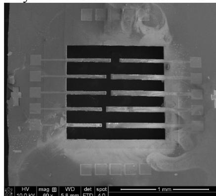
Fig.8 SEM images of released PLZT antiferroelectric microcantilevers
