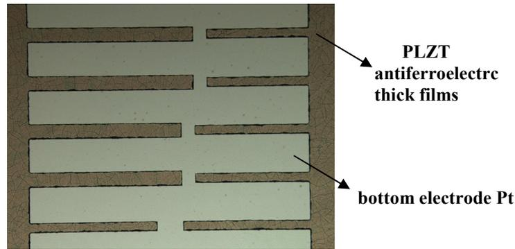
Fig.5 CCD array camera of wet chemical etching for PLZT antiferroelectric thick films
