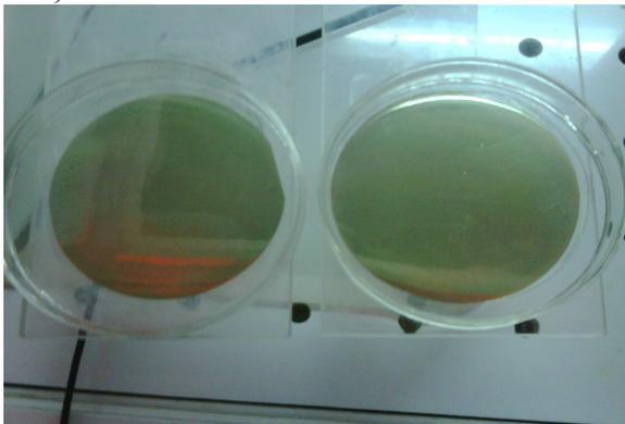
Fig.3 PLZT antiferroelectric thick films deposited on Pt (111)/Ti/SiO<sub>2</sub>/Si (100) substrates
