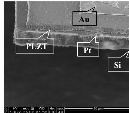
Fig.7 SEM images of side Si-based PLZT antiferroelectric microcantilevers
