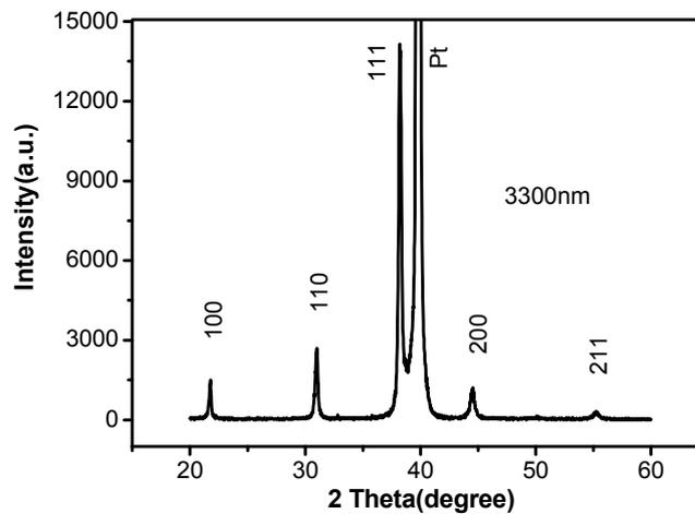
Fig.2 XRD patterns of PLZT antiferroelectric thick films annealed at 700 °C
