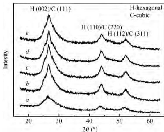
Fig. 1. X-ray diffraction patterns of CdS thin films grown at different temperatures. *a*: 120 °C. *b*: 140 °C. *c*: 160 °C. *d*: 180 °C. *e*: 200 °C.
