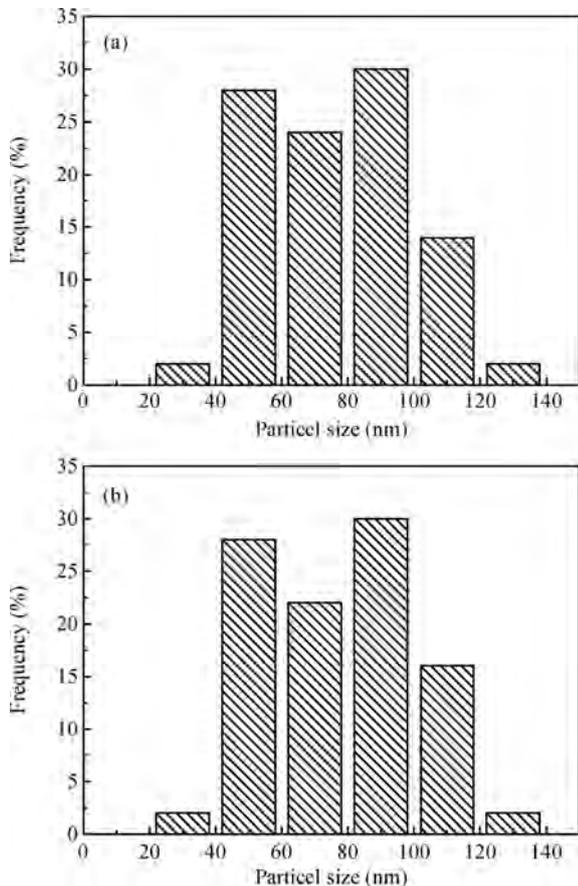
Fig. 5. The histogram of size distribution of CdS thin films grown at different temperatures. (a) 140 °C. (b) 180 °C.
