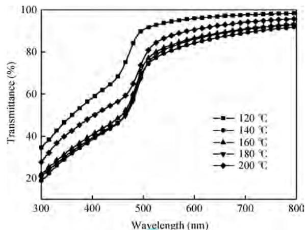
Fig. 6. Optical transmittance of CdS thin films grown at different temperatures.
