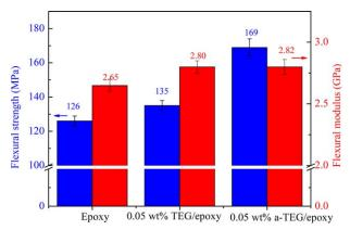
**Figure 9.** Flexural strength and modulus of neat epoxy and nanocomposites. [Color figure can be viewed in the online issue, which is available at wileyonlinelibrary.com.]
