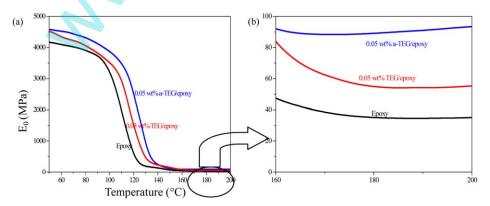
Figure 11. Storage modulus ( $E_0$ ) of neat epoxy and nanocomposites. [Color figure can be viewed in the online issue, which is available at wileyonlinelibrary.com.]
