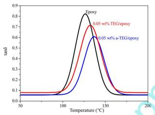
**Figure 10.** Damping factor  $(\tan \delta)$  and glass transition  $(T_g)$  of neat epoxy and nanocomposites. [Color figure can be viewed in the online issue, which is available at wileyonlinelibrary.com.]
