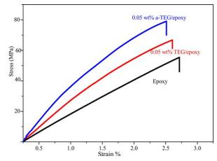
**Figure 7.** Stress–strain curves for neat epoxy, 0.05 wt % TEG/epoxy and 0.05 wt % a-TEG/epoxy. [Color figure can be viewed in the online issue, which is available at wileyonlinelibrary.com.]
