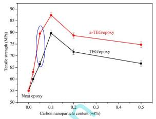
**Figure 6.** Tensile strength and modulus of nanocomposites at different contents of carbon nanoparticles. [Color figure can be viewed in the online issue, which is available at wileyonlinelibrary.com.]
