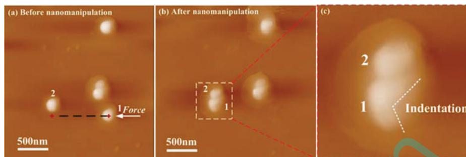
**Figure 4.** Movement of 120 nm polystyrene particles based on vector scanning mode nanomanipulation of atomic force microscope.
