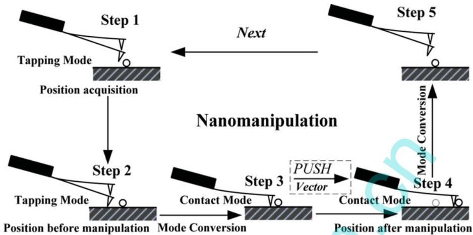
**Figure 1.** Nanomanipulation of nanoobject based on the vector scanning mode of atomic force microscope.
