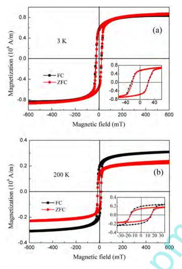
**Fig. 4.** Magnetic hysteresis loops of PSMO/LCMO film at 3 K (a) and 200 K (b) measured after ZFC and FC in 50 mT field. Insets show low field magnetization behavior.
