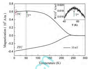
Fig. 2. Temperature dependence of magnetization with ZFC and FC in 10 mT field processes for PSMO/LCMO film. Inset was the enlarged magnetization curves.
