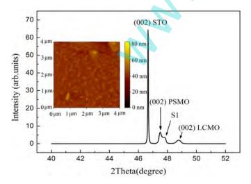
**Fig. 1.** HRXRD  $\theta$ -2 $\theta$  scan centered on the STO (002) peak for PSMO/LCMO bilayer film on (001) STO substrate. Inset: atomic force microscopy contact mode image plotted for an area of 4 × 4  $\mu$ m<sup>2</sup> of PSMO/LCMO film.
