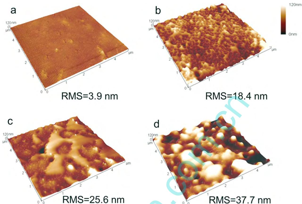
**Figure 3.** Tapping-mode AFM images of the PVC films: (a) PVC film before grafting, (b) PSTG1-grafted PVC film, (c) PSTG3-grafted PVC film, and (d) PSTG4-grafted PVC film. The scan size was  $5 \times 5 \mu\text{m}^2$ . [Color figure can be viewed at [wileyonlinelibrary.com](http://wileyonlinelibrary.com)]
