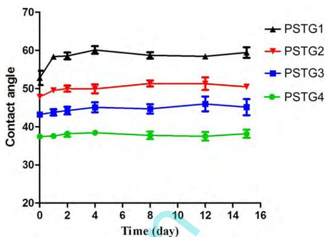
**Figure 5.** Contact angle measurements as a function of time for the PSTG-grafted PVC films. [Color figure can be viewed at wileyonlinelibrary.com]
