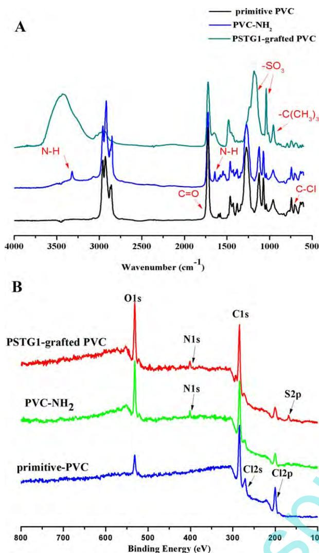
**Figure 4.** (A) ATR-FTIR spectra of the primitive PVC film, amino-functionalized PVC film, and PSTG1-grafted PVC film. (B) XPS spectra of the primitive PVC film, amino-functionalized PVC film, and PSTG1-grafted PVC film. [Color figure can be viewed at wileyonlinelibrary.com]
