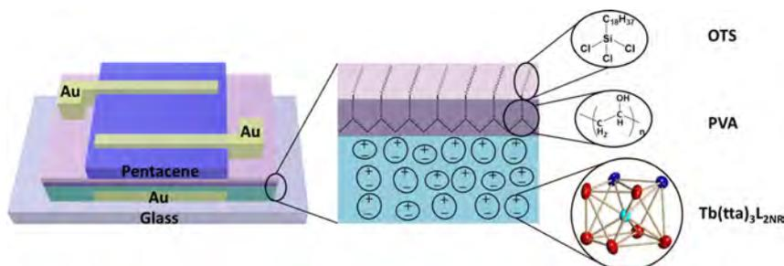
Fig. 1. Schematic diagram of a bottom-gate top-contact OTFTs using pentacene as the channel material and a triple-laminated configuration of  $\text{Tb}(\text{tta})_3\text{L}_{2\text{NR}}/\text{PVA}/\text{OTS}$  as gate insulator.
