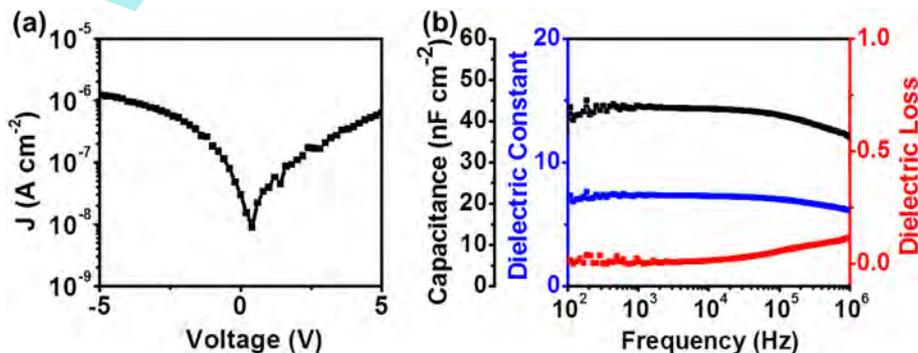
**Fig. 3.** The electrical characteristics of  $\text{Tb}(\text{tta})_3\text{L}_{2\text{NR}}/\text{PVA}/\text{OTS}$  thin film. (a) Plot of leakage current density versus bias voltage of the MIM device. (b) The relationship of dielectric capacitance density, dielectric constant and dielectric loss versus frequency, measured at  $0 \text{ V}$  bias voltage.
