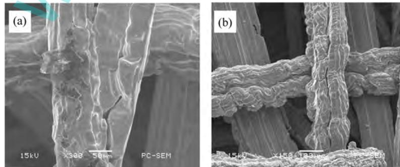
FIGURE 6.—Two kinds of sintering joints between fibers in the PMFSF: (a) fiber-to-fiber contact joints, and (b) fiber-to-fiber mechanical meshing.
