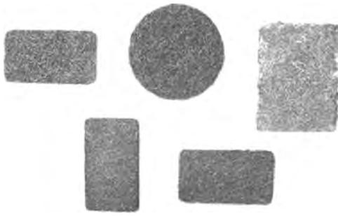
FIGURE 5.—Appearance of the PMFSF with different specified shapes.
