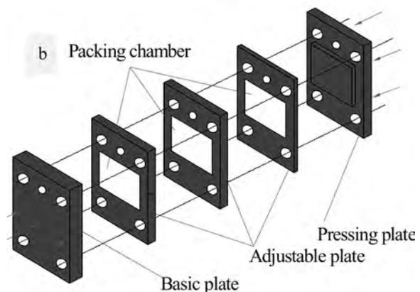
FIGURE 3.—(a) Appearance and (b) assembling principle of the plate-laminated mold-pressing equipment of metal fiber.
