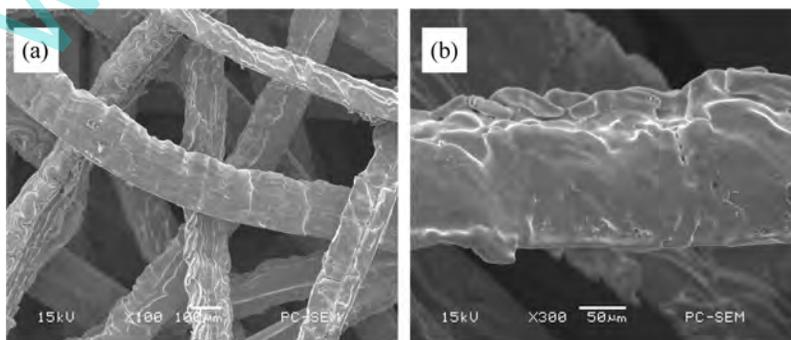
FIGURE 8.—SEM images of (a) the PMFSF (porosity is 80%) and (b) a single copper fiber after sintering at 1000°C for 30 min.
