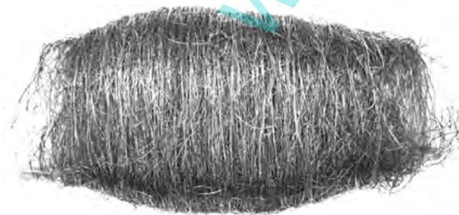
FIGURE 2.—Appearance of continuous fine copper fibers fabricated by the multi-tooth tool.
