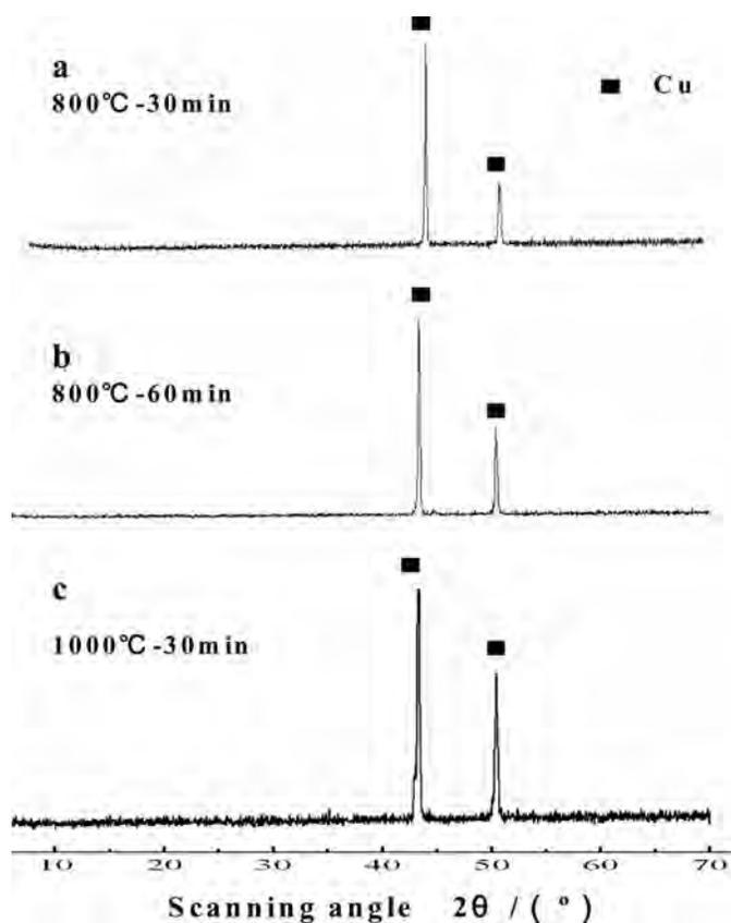
FIGURE 9.—XRD images of the PMFSF sintered under different sintering temperatures and holding times.
