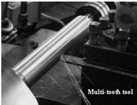
FIGURE 1.—Fabrication process of copper fibers using the multi-tooth tool.
