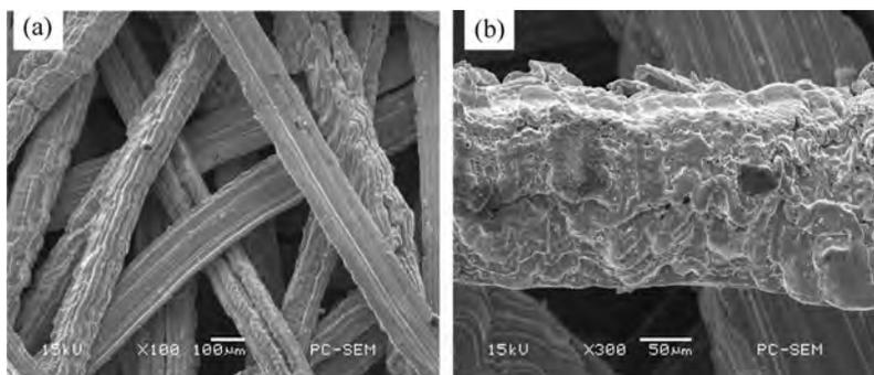
FIGURE 7.—SEM images of (a) the PMFSF (porosity is 80%) and (b) a single copper fiber after sintering at 800°C for 30 min.
