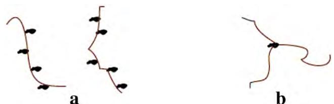
Fig. 5. Effect of PEG amount on TiO 2 colloidal particles (a) lower than critical content and (b) higher than critical content.
