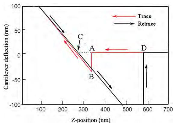
Fig. 3. A typical force–distance plot and schematic illustration for adhesion force calculation.
