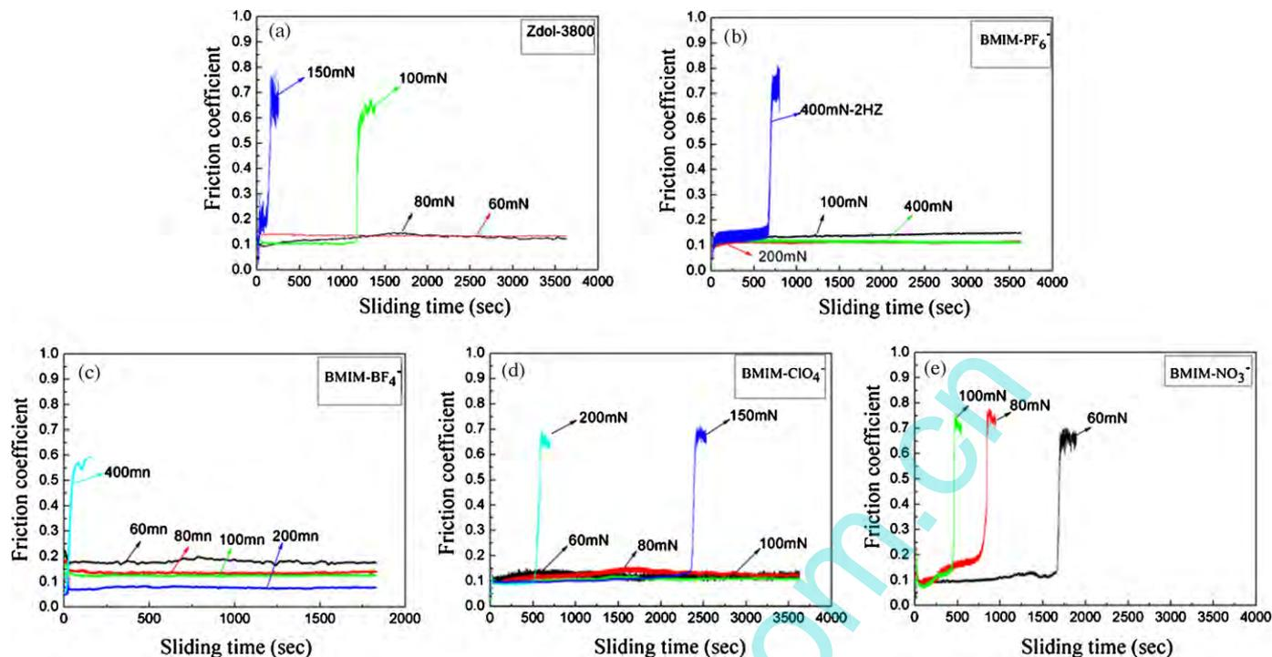
Fig. 8. Friction coefficients as function of sliding cycles for Zdol-3800 (a), BMIM-PF<sub>6</sub><sup>-</sup> (b), BMIM-BF<sub>4</sub><sup>-</sup> (c), BMIM-CIO<sub>4</sub><sup>-</sup> (d) BMIM-NO<sub>3</sub><sup>-</sup> (e), sliding against AISI-52100 steel ball at normal load between 60 and 400 mN and a sliding velocity of 1 Hz.
