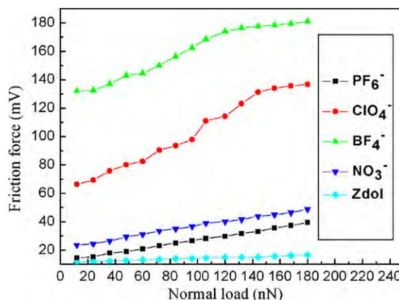
Fig. 7. Nano-friction force versus normal load curves for Zdol-3800, BMIM-PF<sub>6</sub><sup>-</sup>, BMIM-BF<sub>4</sub><sup>-</sup> and BMIM-ClO<sub>4</sub><sup>-</sup>, BMIM-NO<sub>3</sub><sup>-</sup> films at a frequency of 1 Hz.
