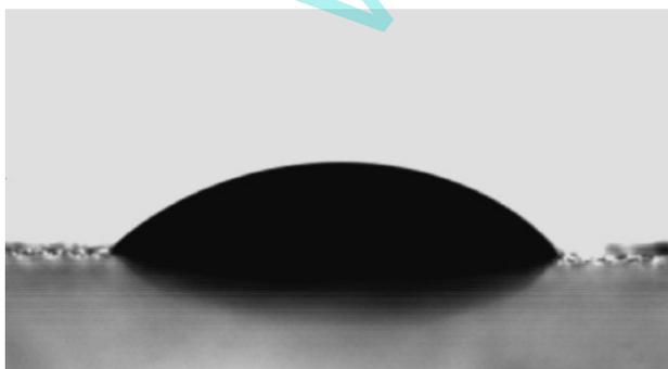
Figure 3. Water contact angle of HLSM.
