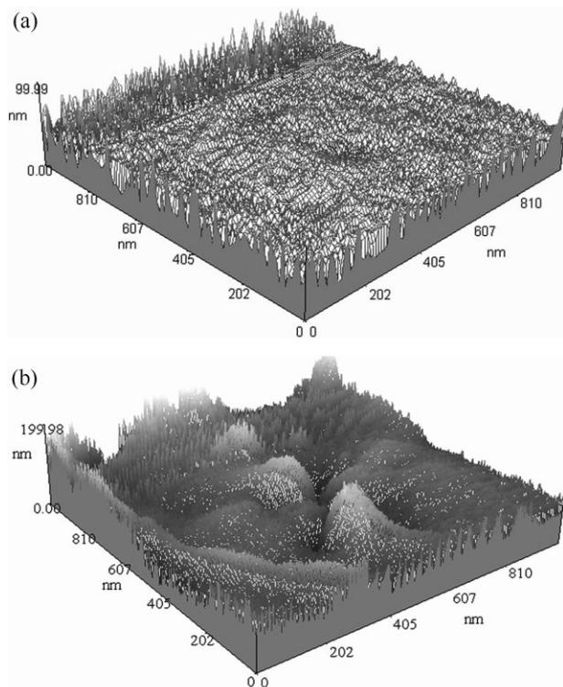
Figure 5. AFM images of PES (FSM-o, a) and modified PES membrane (FSM-5, b).
