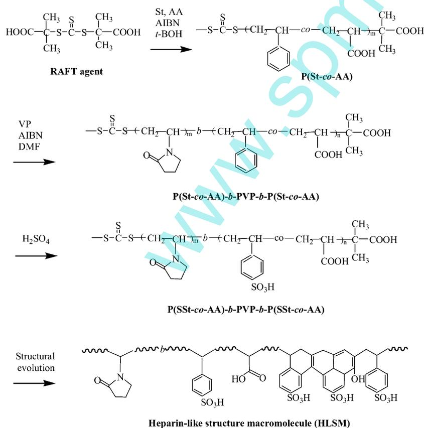
■ Scheme 1. Synthesis of the heparin-like structure macromolecules.
