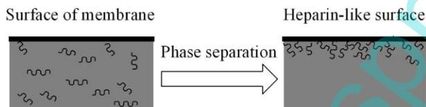
Figure 6. Schematic illustration of HLSM modified membrane formation.
