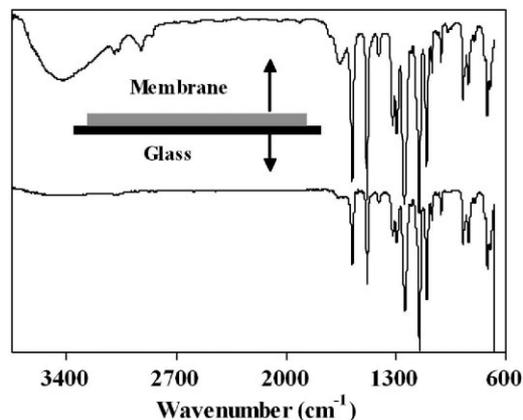
Figure 8. FT-IR spectra for the PES/HLSM membrane surfaces,  $n = 3$ .
