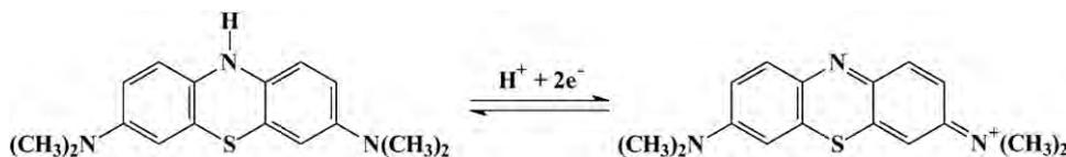
**Scheme 1.** The redox reaction of methylene blue.
