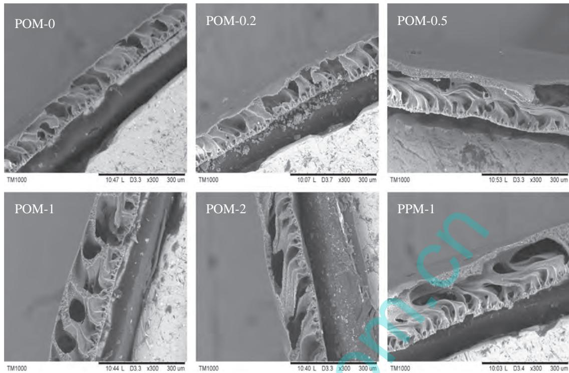
Fig. 4. The cross-section views of membranes with different blend compositions.
