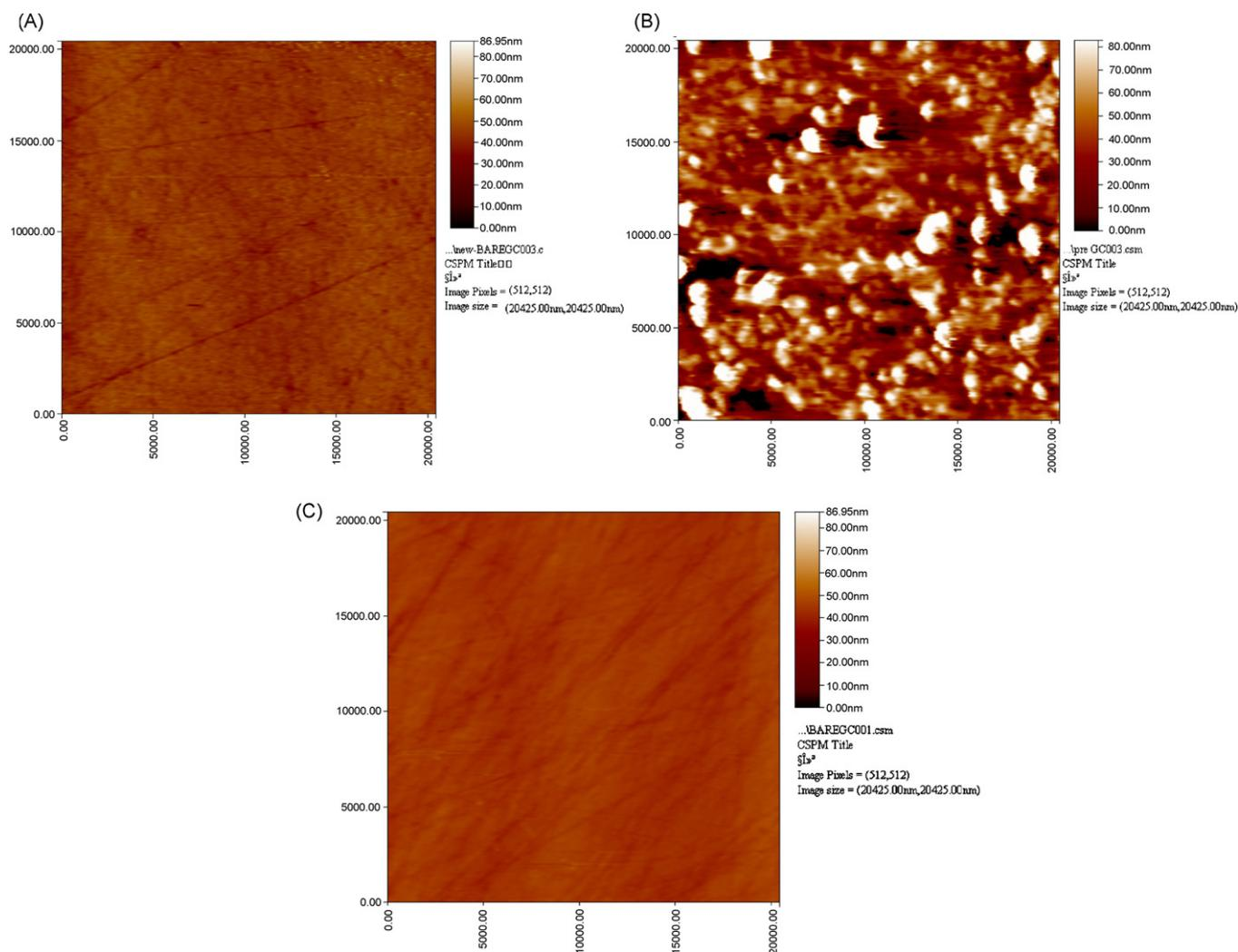
Fig. 2. AFM 2D images of (A) unmodified, (B) oxidized and (C) polished bare GCE.
