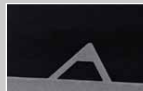
Pyrex-Nitride AFM Probe Triangular Tipless Short Cantilever Close-up
