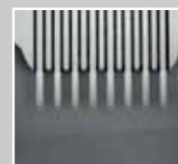
Arrow™ TL8 Tipless cantilever array, eight cantilever beams on a single crystal silicon support chip
