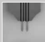
Arrow™ TL2 Tipless cantilever array, two cantilever beams on single crystal silicon support chip
