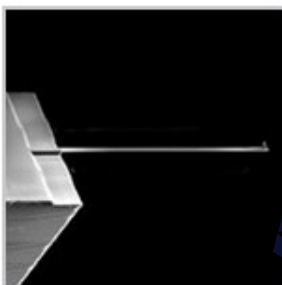
SEM image of Silicon cantilever and probe.
